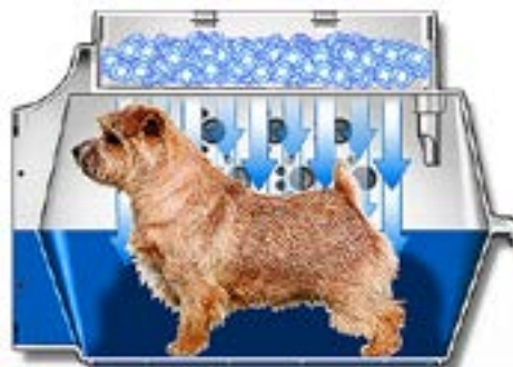
2. STANDARD CONVECTION CAUSES COLD TO FALL
